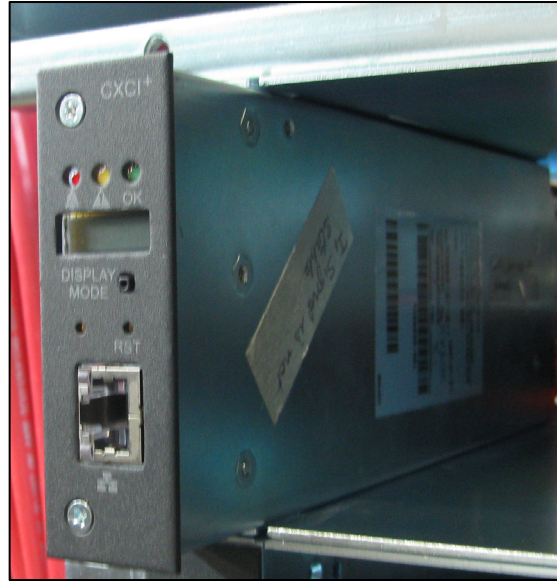
Figure 5—Showing CXCI+ controller module installation
