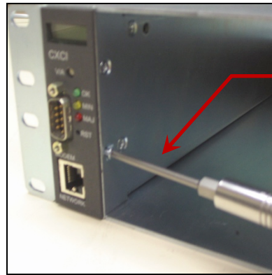
Figure 8—Showing CXCI module installation
